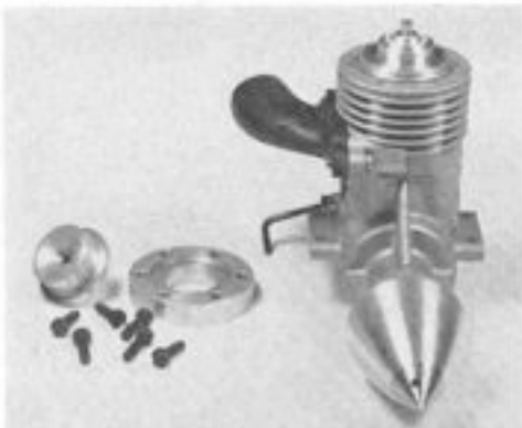
Picture shows the modified Cox head within its adaptor placed in position. The modified cylinder head (seen alongside with a modified Cox head) clamps this new unit in position.
